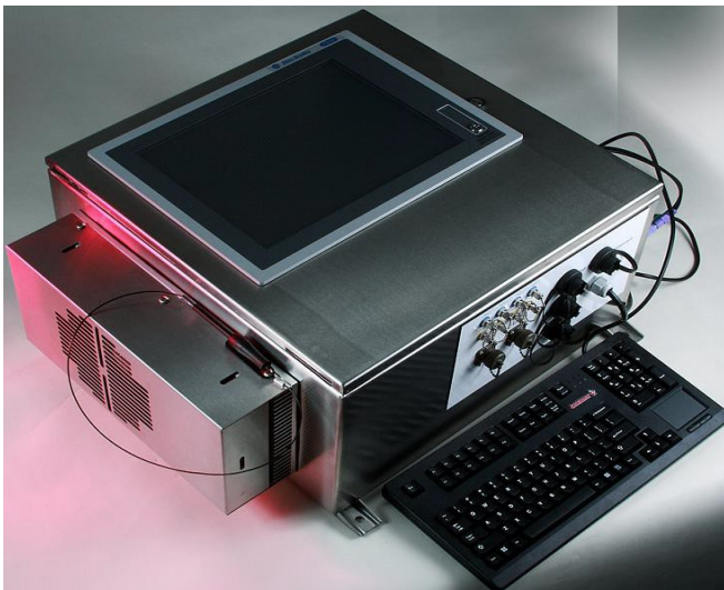
Photo 2: ICS stainless steel NEMA4 box with touch-screen
