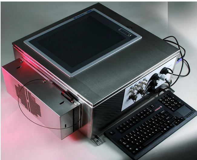
Photo 4: Stainless Steel NEMA4 box with touch-screen
